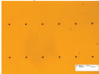
Fig.4 Seed layer deposition with 4.5um diameter and 40um depth TSV
